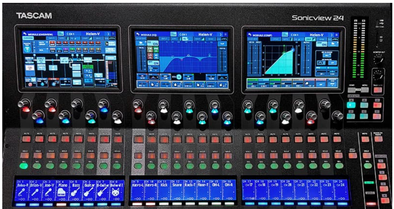
Top surface detail of the console’s three 7” touch screens; illuminated select, mute and solo buttons; and LCD name strip displays on each channel. The color LEDs below the rotary encoders change to indicate their function for each selected screen. Photo by author.
