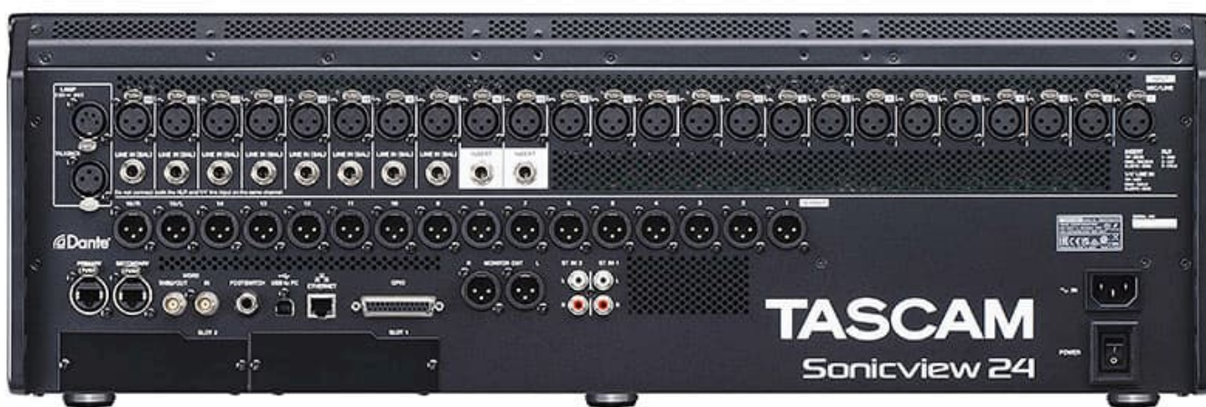
The rear panel reveals the 24 input channels, 16 balanced outputs, onboard Dante interfacing, GPIO, two expansion slots and more
