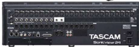
The rear panel reveals the 24 input channels, 16 balanced outputs, onboard Dante interfacing, GPIO, two expansion slots and more
