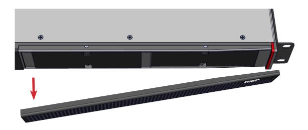
3. Use the lifted side to remove the grille from the device and proceed to the cleaning the filter steps on page 14.
