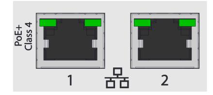
Connect network port 1 to a PoE+ switch to enable quick recovery of audio when the mains supply is temporarily lost. Audio from the device, including from the analog inputs, is not available while the device is powered from PoE+. Powering the device requires a compliant PoE+ class power source or above.
