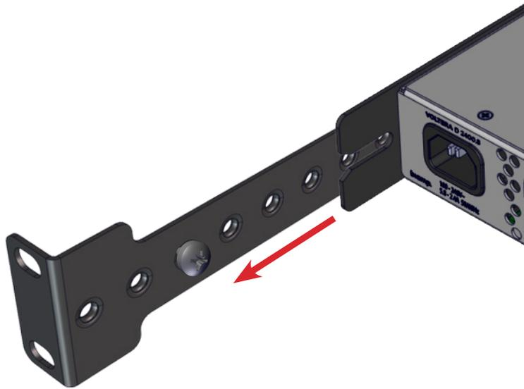
5. Secure the mounting plate to the server rack.
