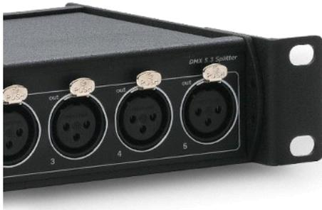
The Martin DMX 5.3 Splitter is the most economical protection for DMX controllers and devices. The main purpose of the Martin 5.3 Splitter is to maintain proper data over long or several runs of DMX signal. The Splitter boosts the weak DMX signal to its original output level before it becomes too low to be read from DMX devices. Disruption of DMX is often caused by bad cables or bad connections. The Martin DMX 5.3 Splitter will help to rectify the signal.
