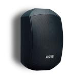
The MASK4T loudspeaker has a unique innovative design and its transparent sound offers incredible intelligibility ideal for background music and paging purposes. MASK4T can be used in low impedance 16 ohms (up to 4 loudspeakers in parallel on a standard 4 ohms amplifier channel) or in 100 volt with several power tappings (20 - 10 - 5 - 2.5 watts).
