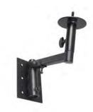
This wall bracket can be used with our MASK12 speaker or other compatible speakers up to 40 kg. To install the MASK12 speaker on the bracket, remove the center M10 bolt from the bottom of the speaker. Attach the pole mount (supplied) securely by fastening the mount on the speaker. The speaker arm can be swiveled over a 180° angle from left to right and can be tilted down up to 20° by turning the tilt screw.
