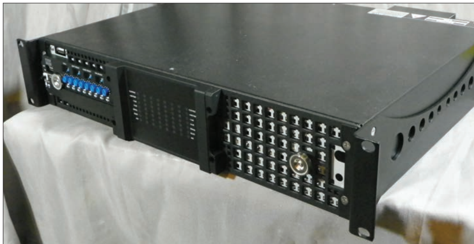
Powersoft Ottocanali front panels removed, showing the blue input attenuators and other controls on the left side. The magnetic disks on either side help to secure the panels.
