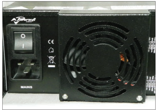
Rear panel cooling fan plus mains connector and power switch.
