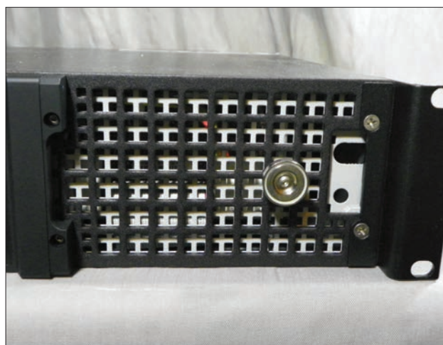
Cooling vent intake.
