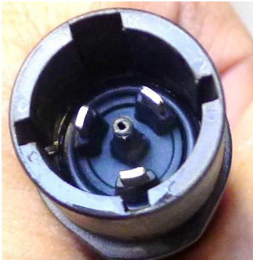
After IP65 test: No water and no dust entered
