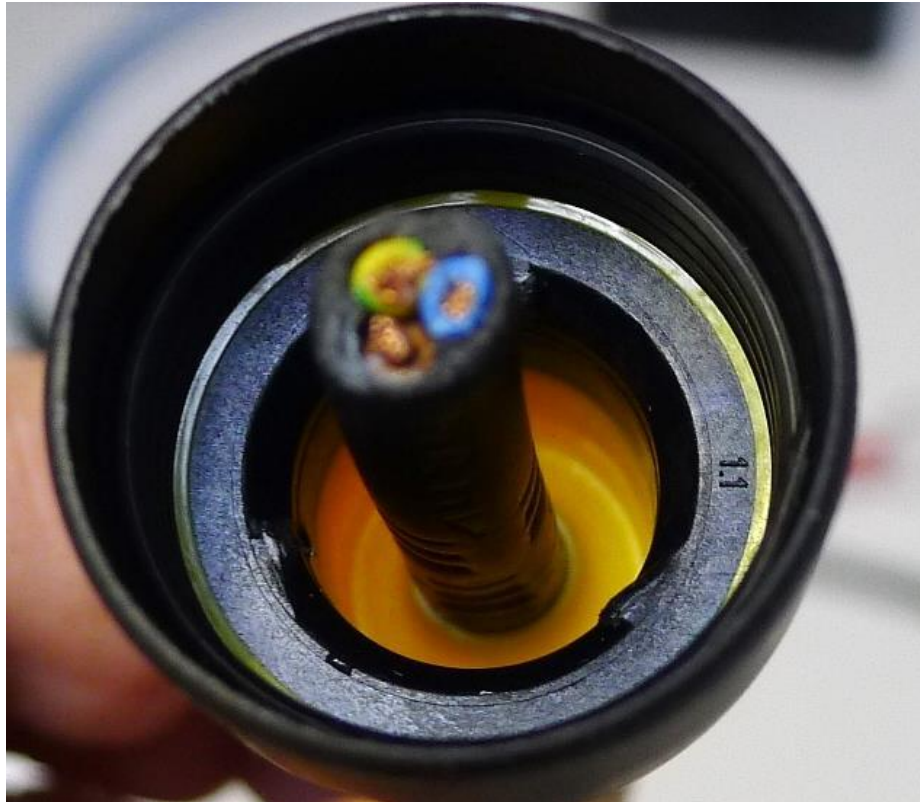
After IP65 test: No water and no dust entered
