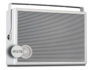
The SMB6VP is a functional cabinet speaker with mounting bracket. It has a 5" paper woofer, and is equipped with a 100 volt power transformer with power taps on 1.5 - 3 - 6 watts.
