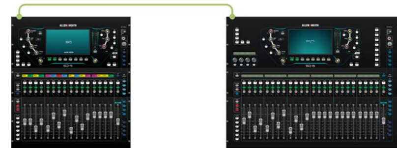
SQ to SQ direct 96kHz connection using gigaACE Send and receive all assignable I/O
