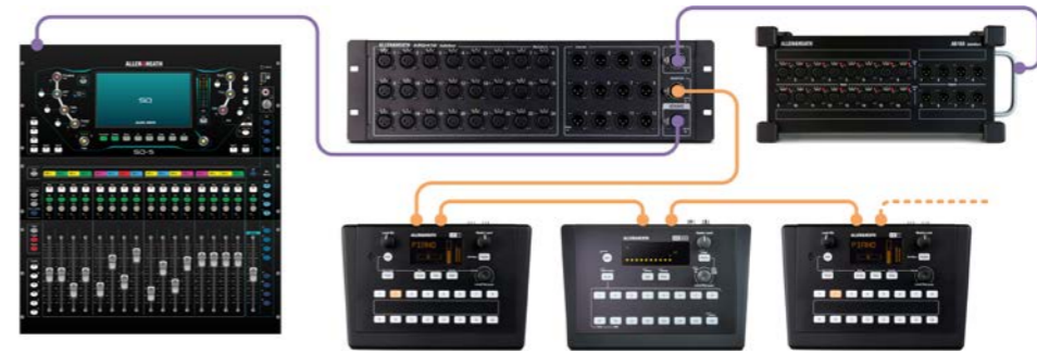
SQ expanded using AR2412 + AB168 40 remote inputs + 20 remote outputs + ME system
