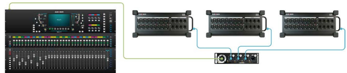
SQ expanded with 3x DX168s connected to a DX-Hub for full 96kHz operation, 48 remote inputs and 24 remote outputs
