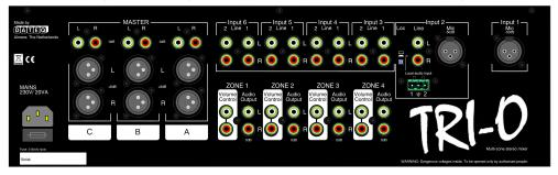
Channel 1 has a talk-over circuit to improve the speech intelligibility. This circuit, which is triggered by the microphone signal from channel 1 (i.e. it is voice-activated), ensures that this signal overrides all others. The talk-over function can be disabled with the TalkOver switch on the front.
