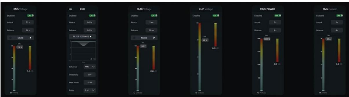
**Detailed limiter functions** with RMS, peak and clip limiters as well as a current and true power limiter. In addition, a dynamic EQ is also included; the filter's gain is controlled by the signal level (Fig. 4)
