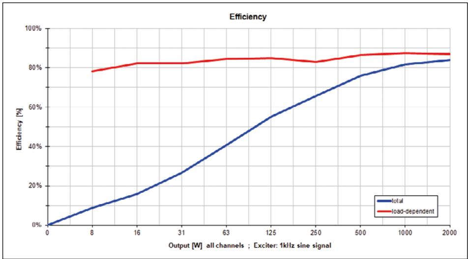
**Efficiency as a function of output power** The blue curve refers to the total power, the red curve refers to the load-dependent share without base load (Fig. 23)
