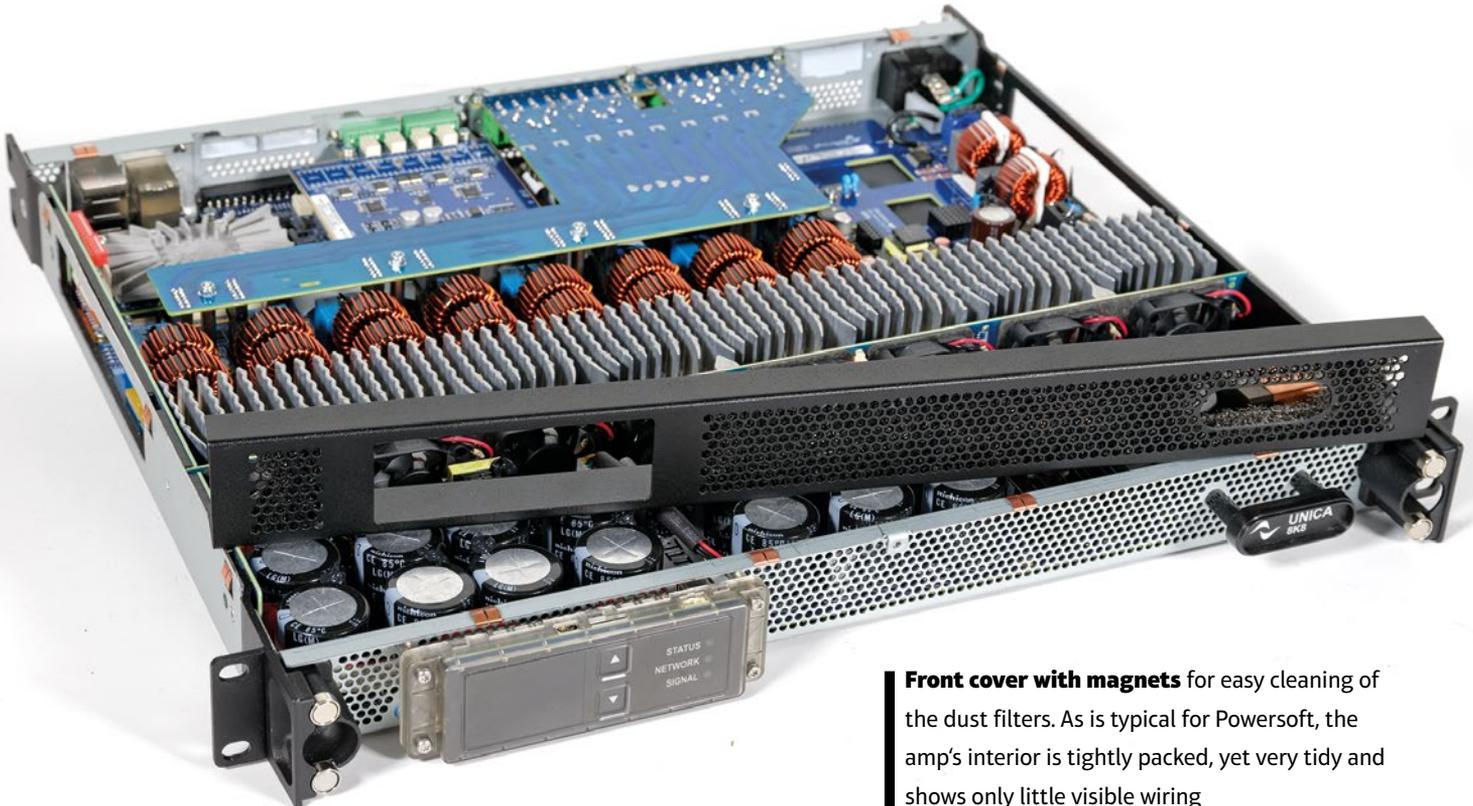
**Front cover with magnets** for easy cleaning of the dust filters. As is typical for Powersoft, the amp's interior is tightly packed, yet very tidy and shows only little visible wiring
