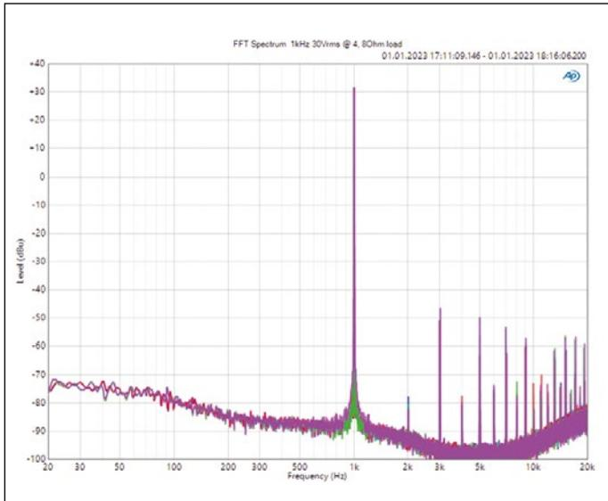
**Exemplary distortion spectrum** for channels 1 and 2 at an output voltage of 30 V<sub>rms</sub> with a load of 4 Ω (red, blue) and of 8 Ω (green, purple). All distortion components are located below -80 dB (0.01%) and therefore completely uncritical (Fig. 14)
