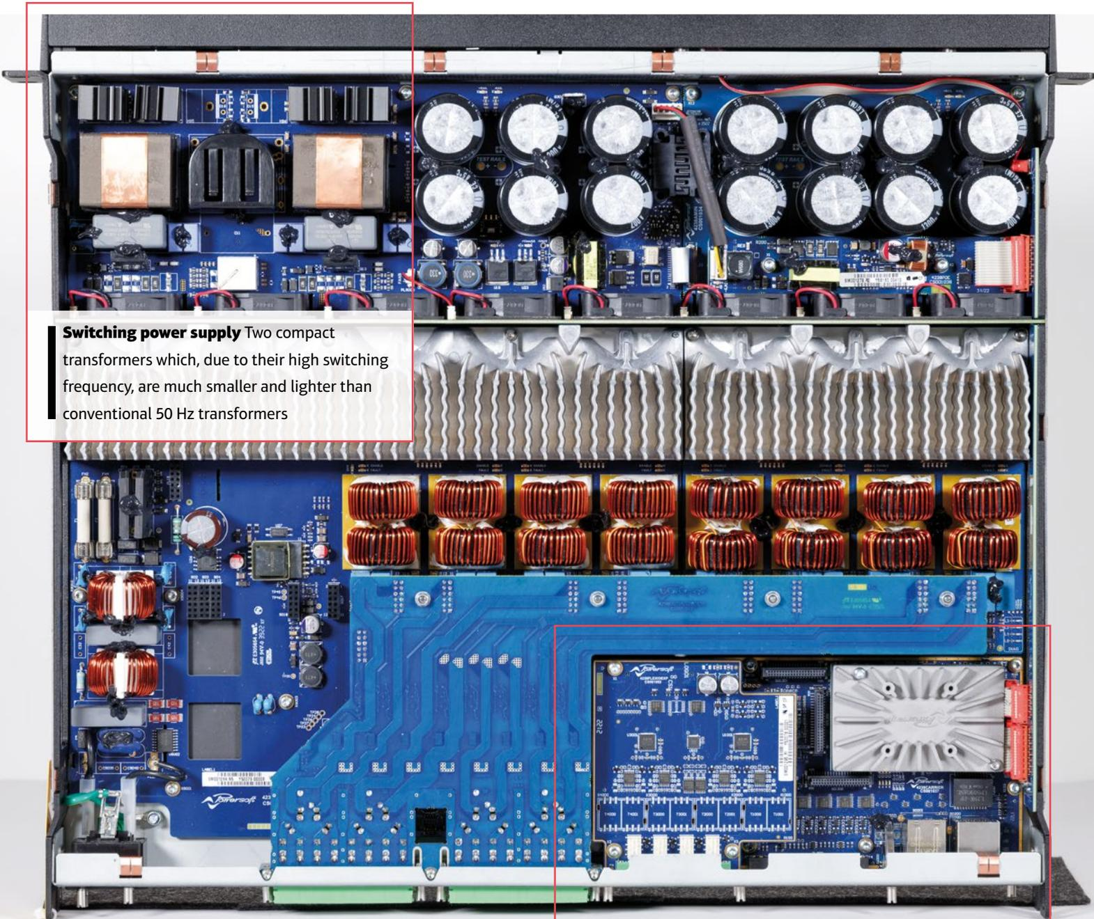
**Switching power supply** Two compact transformers which, due to their high switching frequency, are much smaller and lighter than conventional 50 Hz transformers
