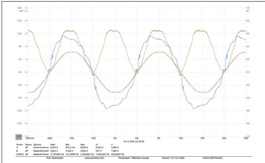
**Power Factor Correction** Course of mains voltage (red), mains current (blue) and calculated power consumption (green). The PFC performs very well (Fig. 24)
