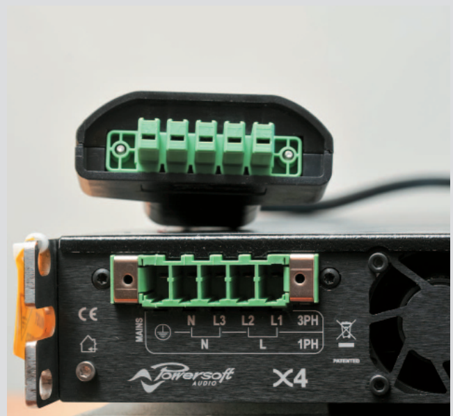
3-phase connection with a large 5-pole Euroblock Phoenix connection. Depending on requirements, both amplifiers can be operated with one, two or three phases.
