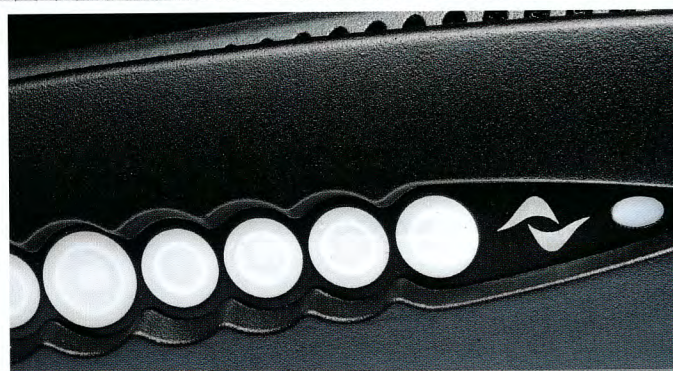
A central on-off button is flanked by LED push buttons representing each channel
