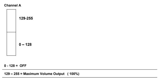
The Z-1020 fog machine has onboard DMX control. Currently this model uses 1 channel to control volume output operation. Each channel has a value range of 0 to 255. On/Off function can be programmed using the DMX controller or the DMX control software being used by lighting and effects operator.
