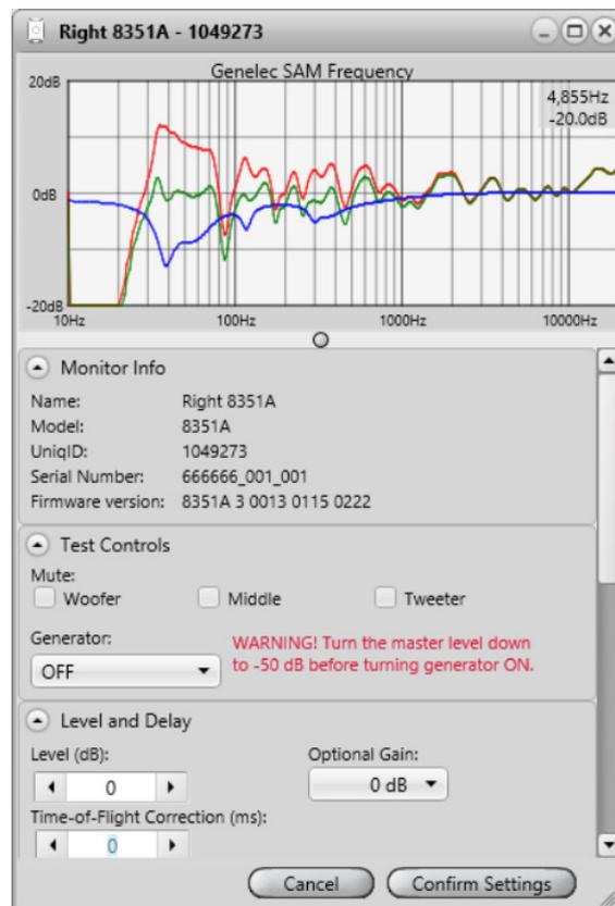
Figure 26. Example of the acoustical calibration editor window
