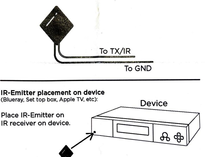
Clear adhesive layer placed toward device (Replace, if necessary, with supplied 2-sided tape)
