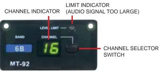
The module transmitter MT 92 cannot be updated via IR. Channel selection takes place manually by pressing the CH button The transmitter can be switched on and off by a long press of the CH button.
