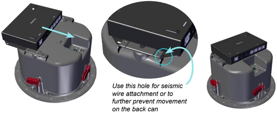
3. A cover is provided for conduit usage. Punch out and feed wiring through the opening, and connect per the device instructions. Insert tabs into the slots on the Tesira unit and tighten the thumb screw to secure the cover to the C-IC6 enclosure.
