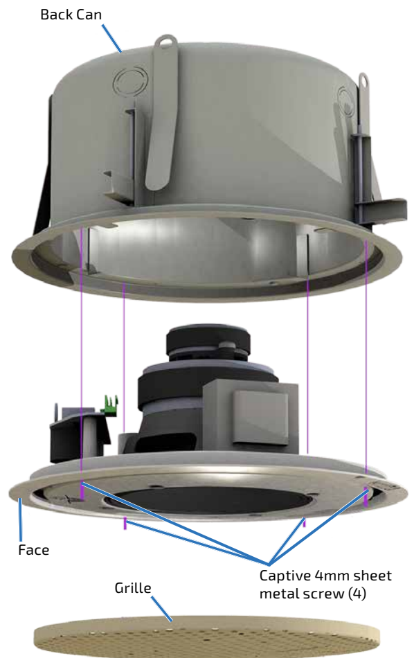
Figure 15. Use the four included, captive, 4mm sheet metal screws to secure the loudspeaker into the can. Use the screws after inserting loudspeaker into the back can and twisting to retain it.
