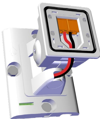
Figure 2. Wire path to wire the ClickMount bracket (single wire shown)
