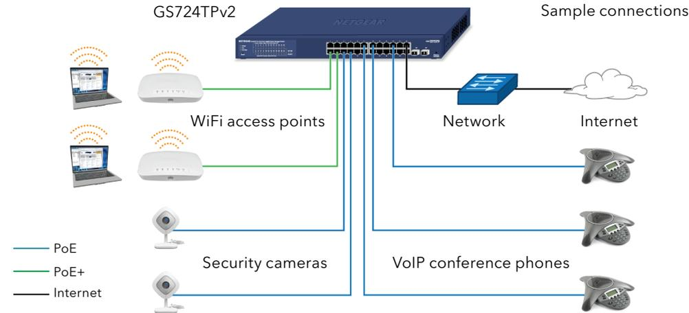
1. Connect devices to the RJ-45 PoE+ network ports on the switch front panel. Use Category 5e (Cat 5e) Ethernet cables terminated with RJ-45 connectors to make Gigabit connections.
