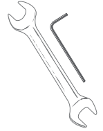
Figure 3-4. Fully tighten all connections before lifting
