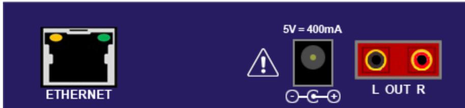
! With an RCA to female jack converter cable the RCA connectors can also be used for headphones.
