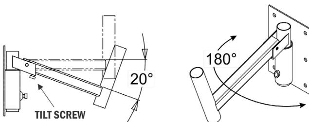
For additional safety, we strongly advise to secure the speaker using a safety chain. The chain and the necessary mounting hardware(eyebolts) are not supplied with this bracket. The chain and the attachment eyebolts should be capable of supporting 12 times the weight of the speaker. Mount the safety chain in such a way that the speaker or the supporting hardware won't drop more than 20 cm.
