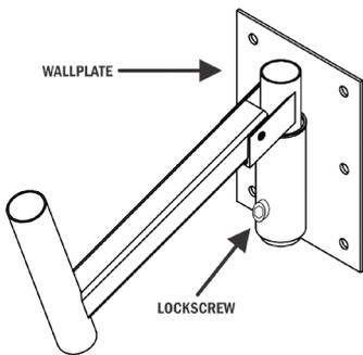
Fix the wall plate on a sufficiently strong wall using all 6 mounting holes. Always use mounting hardware (not supplied) capable of supporting the load safely. The speaker arm can be swiveled over a 180° angle from left to right and can be tilted down up to 20° by turning the tilt screw. Mount the speaker with the attached speaker pole mount on the bracket and secure it by tightening the lock screws.
