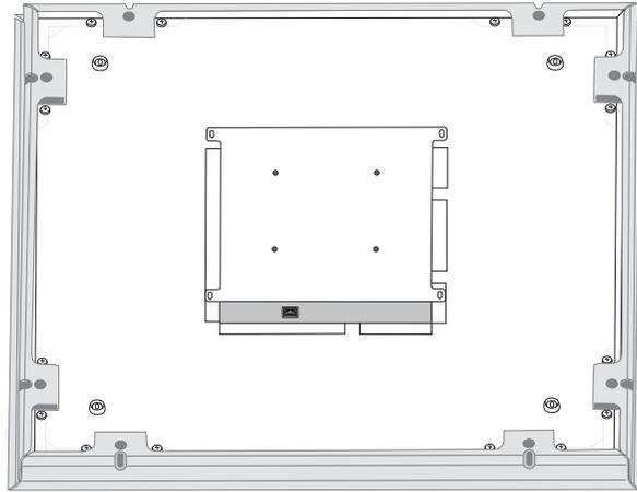
Screw the adapter pieces on as shown, using 2 screws per side.
