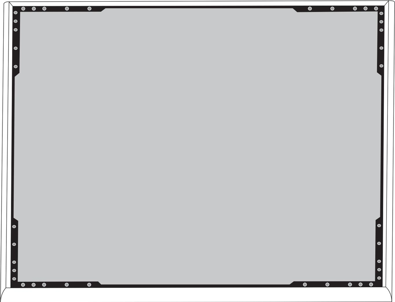
(2.1) Masking off the extrusion (highlighted in black)
