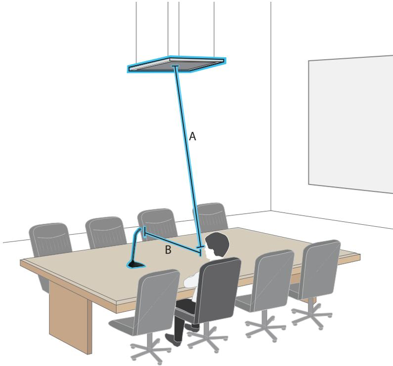
In this example, the acoustic performance of the array microphone mounted (A) feet from the talker matches the cardioid gooseneck microphone placed at a distance of (B) feet from the talker.
