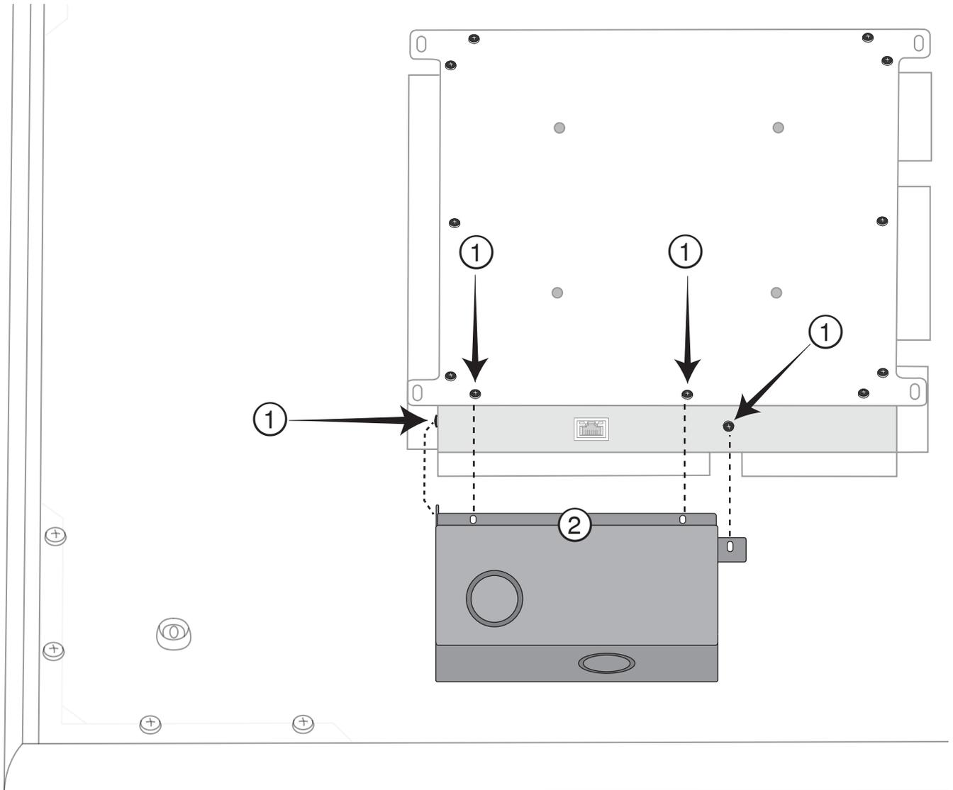
3. Install the 4 screws to secure the junction box on the microphone.
