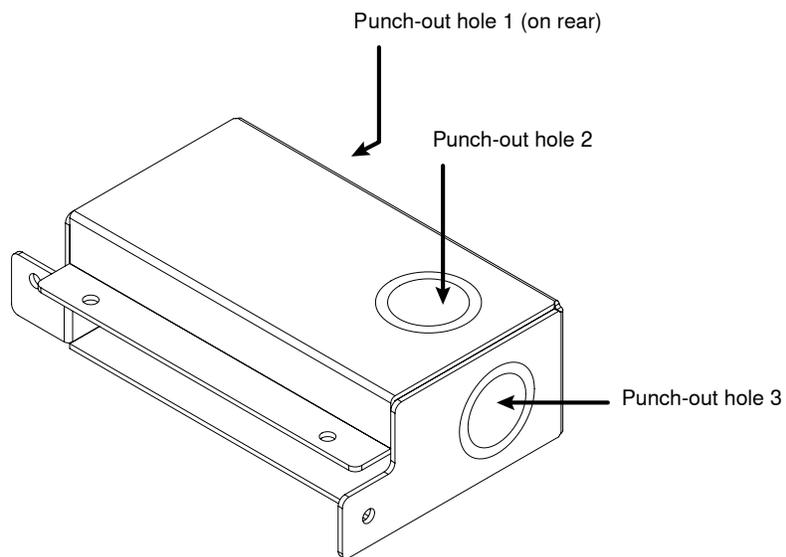
**Important:** Punch out the necessary holes in the junction box prior to installing it onto the microphone.
