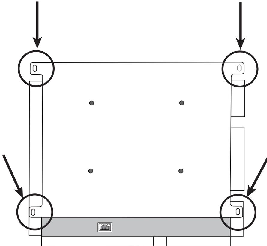
Attach a safety tether between the building structure and one of the tie-off points on the back panel of the microphone. This safety measure prevents the microphone from falling in an emergency situation. Make sure there is no tension on the safety tether to ensure the microphone is resting properly in the ceiling grid.
