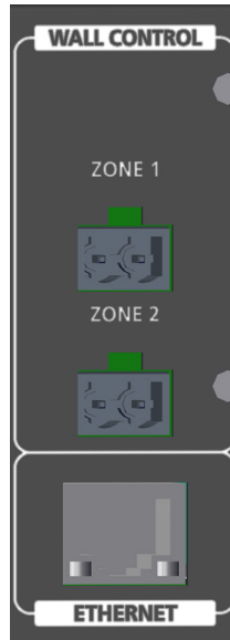
Figure 8. Wall Control & Ethernet
