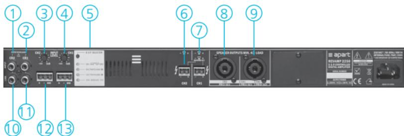
1. **Channel 2 overload led:** when this led lights up, you are overloading the input. Lower the input signal immediately to prevent the amplifier from shutting down.
